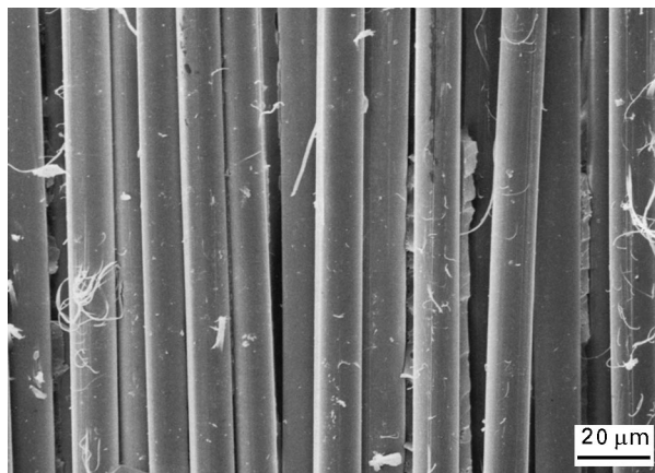
Figure 3 Scanning electron micrograph of the shear fracture surface of an untreated aramid/Resinox® CL1579 composite sample autoclave cured with 4% acid catalyst for 1 h at 60 °C, 2 h at 80 °C and 1 h at 120 °C, showing clean fibre/matrix separation, indicative of weak interfacial bonding.
